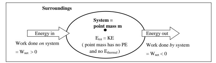
The 1<sup>st</sup> Law applied to a simple mechanical system.
