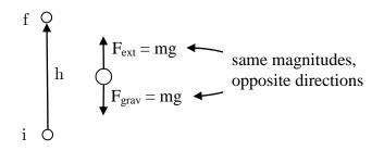
So  $W_{ext} = +mgh$  and  $W_{grav} = -mgh$ . This is true for the special case  $\mathbf{v} = constant$ , but it turns out that it is always true that  $W_{ext} = -W_{grav}$ , regardless of the motion, so long as the KE at the final position is the same as the KE at the intial position. So,  $W_{ext} = -W_{grav}$ , if the mass starts and finishes at rest:  $v_i = v_f = 0$ . With this example in mind, we are ready to define PE.
