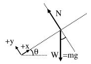
For N-II, we'll want the components of the forces. Look at the force diagram. The Normal force N is easy, by inspection:  $N_x=0$ , and  $N_y=+N$ .
