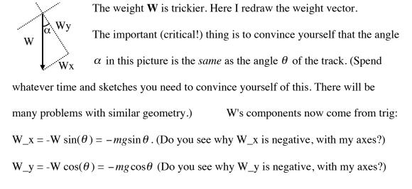
We're all set up. Write out N-II in the x- and y- coordinates:
