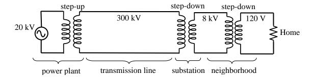
A very simplified model of power distribution (transformers not shown):
