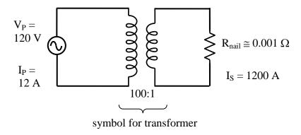
Power dissipated in nail =  $I_S^2 R = (1200)^2 (10^{-3}) = 1440 W \implies \text{will melt nail.}$
