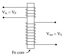
Secondary coil = output coil, with  $N_S$  turns
