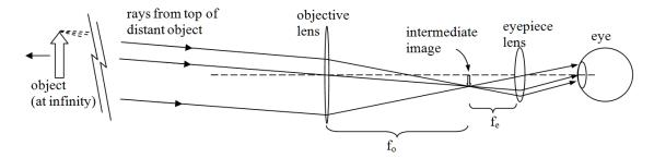
In this diagram, the rays entering the objective lens represent rays from the topmost point of the distant object. The rays exiting the eyepiece lens are parallel rays, which are about to enter the observer's eye.
