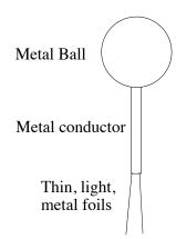
You can NOT tell what the sign of the net charge on the electroscope is simply by looking at it: If it's net +, the foils repel. If it's net -, the foils repel! So, all you can do is see HOW charged it is.
