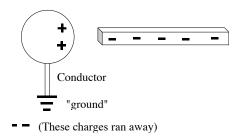
Electrons are free to run along conductors, and they can get much farther away by going to the ground. So they do! (Interestingly, it doesn't matter WHERE exactly you touch the conducting wire to the ball: if you give those electrons a chance to run away, they'll take it.)
