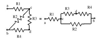
If I asked for the "equivalent resistance" between a and b in the above two, the one on the left looks scary.
