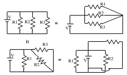
All those circuits are just 3 resistors in parallel. I personally prefer the first drawing, because it makes it visually obvious that the voltage V across all 3 resistors is exactly the same. (Like 3 parallel runs down the ski hill) By the way, this setup is pretty much how houses are wired up for appliances: here's one MORE drawing, which is pretty much equivalent to all the ones above:
