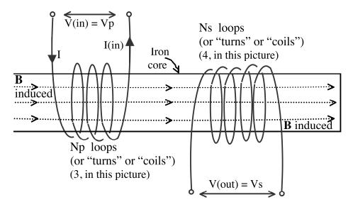
If V(in) is steady (I(in) is steady) then **B**(induced) through the coils is steady. The flux  $\Phi$  through the secondary coil is therefore steady, and Faraday's law says V(out)=0: *no output current, or voltage*.
