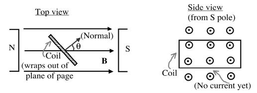
We've seen this setup before, in Ch. 20. (Remember, if you run a current I through that coil of wire, RHR #2 says there are forces that twist the loop. That's a MOTOR, putting current into it causes mechanical motion.)
