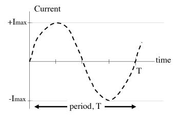
The frequency is exactly the same as the mechanical frequency of the rotating loop. In the US, that means you must turn that loop 60 times/sec, or 60 Hz.
