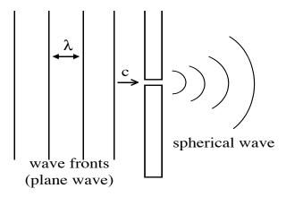
Each point on *any* wavefront can be considered to be the source of a new outgoing spherical wave.
