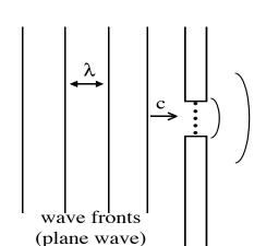
With a wider gap, each point in the gap acts as a point source. Each of those points emits spherical waves!
