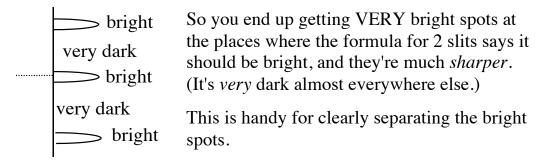
We call a device like this, with many slits, a **diffraction grating**.
