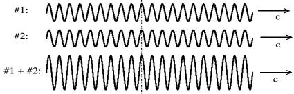
If they are "in phase" (meaning, the peaks are lined up) and if the waves are traveling at the same place and time, they will add up, they **superpose**, as waves always do. The resulting wave, the sum of the two, has the same f, c, and direction, but *twice* the amplitude. The waves have **constructively interfered**.
