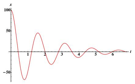
You can obtain an estimate for  $\omega_1 = \sqrt{\omega_0^2 - \beta^2}$  using the time between successive zero crossing. Estimate  $\omega_1$  in the figure above and explain how you obtained your result.
