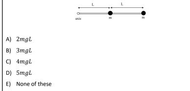
A light rod of length 2L has 2 small heavy masses (each with mass m) attached at the end and the middle. The fixed axis of rotation is at the left end, as shown. If the bar is released from rest, what is the magnitude of the initial angular acceleration?
