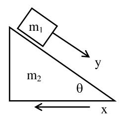
CT15-7. A block of mass  $m_1$  slides on an inclined plane of mass  $m_2$ . The equations of motion are
