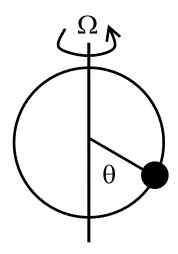
CT15-3. A bead of mass m slides on a circular wire of radius R. The wire rotates about a vertical axis with angular velocity  $\Omega$ . When the bead is at angle  $\theta$ , what is the  $\theta$  component of the centripetal force on the bead?
