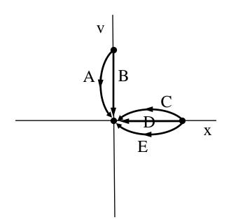
CT4-11. What kind of damped undriven simple harmonic oscillator does this phase path show?
