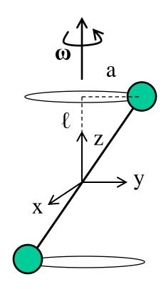
Consider the body frame aligned with the principle axes of inertia (as sketched). What are the components of the angular velocity vector in this frame?  $\begin{bmatrix} & & & \\ & & & \\ & & & \\ \end{bmatrix}$
