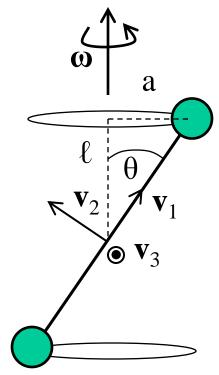
Consider the body frame aligned with the principle axes of inertia (as sketched). In this frame, the torque is constant in the 3 direction (out of the page). How can you describe the torque in the space frame?
