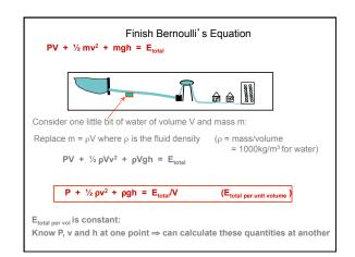
Here I have a tank of water with a hose connected to the bottom. When I take my finger off the hose, water (under pressure) will squirt into the air. Will the water go higher or lower than the opening in the tank (dashed line)?
