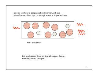
can get amplification, but to really build up to nice high power beam need feedback of mirrors.
