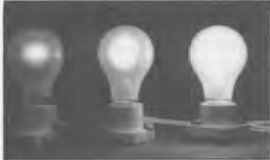
Fig. 6.3.1 - As you increase the power to an incandescent light bulb, its filament becomes hotter and emits a brighter and whiter light. The cooler filament on the left is dim and red while the hotter one on the right is bright and yellow-white.
