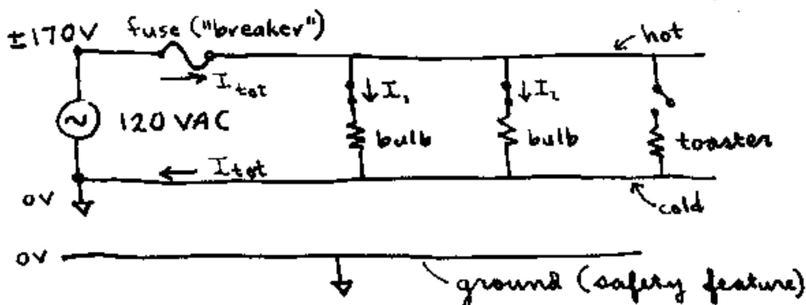
If  $I_{tot} > 15A$ , breaker opens, preventing wires from over-heating
