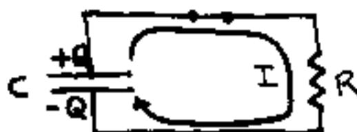
$$\text{At } t = 0^+, I_0 = \frac{V_0}{R}$$
