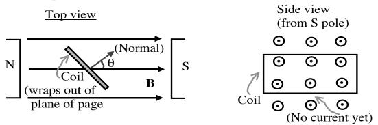
We've seen this setup before, in Ch. 29. (Remember, if you run a current I through that coil of wire, RHR #2 says there are forces that twist the loop. That's a MOTOR, putting current into it causes mechanical motion.)
