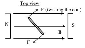
The flux through the coil,  $\Phi = B A \cos\theta$ , is *changing*, because  $\theta$  is now steadily changing.
