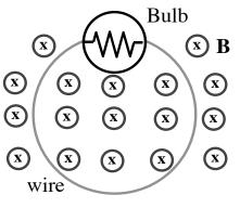
Imagine a **B** field whose field lines "cut through" ("pierce") a loop. Define  $\theta$  as the angle between **B** and the "normal" or "perpendicular" direction to the loop.
