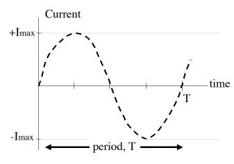
The frequency is exactly the same as the mechanical frequency of the rotating loop. In the US, that means you must turn that loop 60 times/sec, or 60 Hz.
