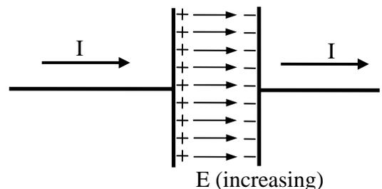
that he could fix the problem by modifying Ampere's Law with the addition of a new term. The changing electric flux in the capacitor leads to a quantity that has the
