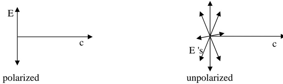
Polarizer = polaroid filter = filter that passes light with the  $\mathbf{E}$ -field along the "pass axis" of the filter.
