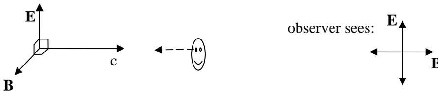
Ordinary light (from the Sun or a lightbulb) is unpolarized, a mixture of waves with E-field in random directions but always  $\perp$  direction of travel.
