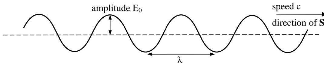
Consider a small source of monochromatic (single-wavelength) light, emitting energy at a rate  $P$  (in J/s). If the source sends light out in all directions uniformly, then the *wavefronts* are expanding spherical shells. A small detector (like an eyeball), very far from the source, will sense a small portion of the wavefronts. Over the small region that is detected, the wavefronts are nearly flat planes. Such a beam of light is called a *plane wave*.
