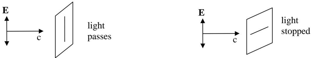
If  $\mathbf{E}$  is not parallel to the pass axis, then only the *component* of  $\mathbf{E}$  along the pass axis gets through.
