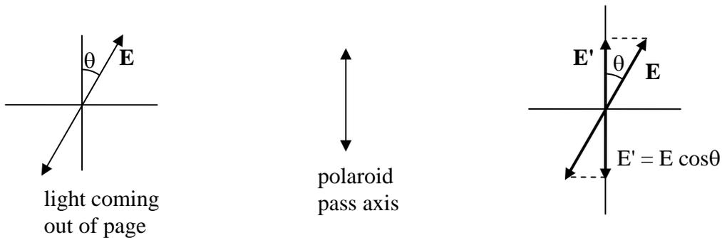
The intensity of the light is proportional to  $E^2$ , so  $I_{\text{trans}} = I_0 \cos^2 \theta$ .
