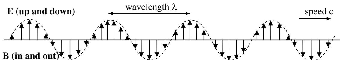
All EM radiation is caused by shaking (accelerating) electric charge. The more rapidly the charge is shaken (the higher the frequency of the shake), the shorter the wavelength of the light, since  $\lambda = \frac{c}{f}$ . Now we can understand why all things glow (give off light) when they get hot.
