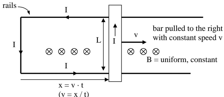
The bar+rails form a wire loop of area  $A = L \cdot x = L \cdot v \cdot t$ . The magnetic flux  $\Phi = B \cdot A$  is increasing, which produces an emf, which drives a current  $I$  (an eddy current!) which is CCW by
