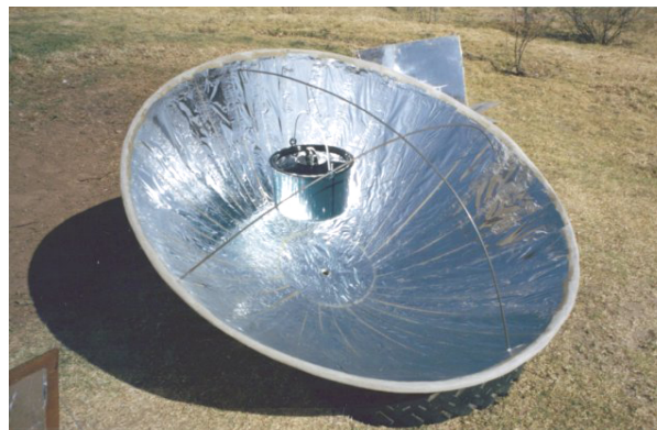
Concave solar concentrator
