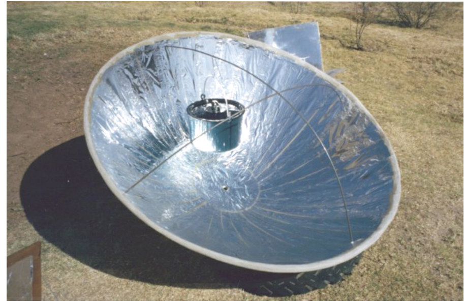
Concave solar concentrator
