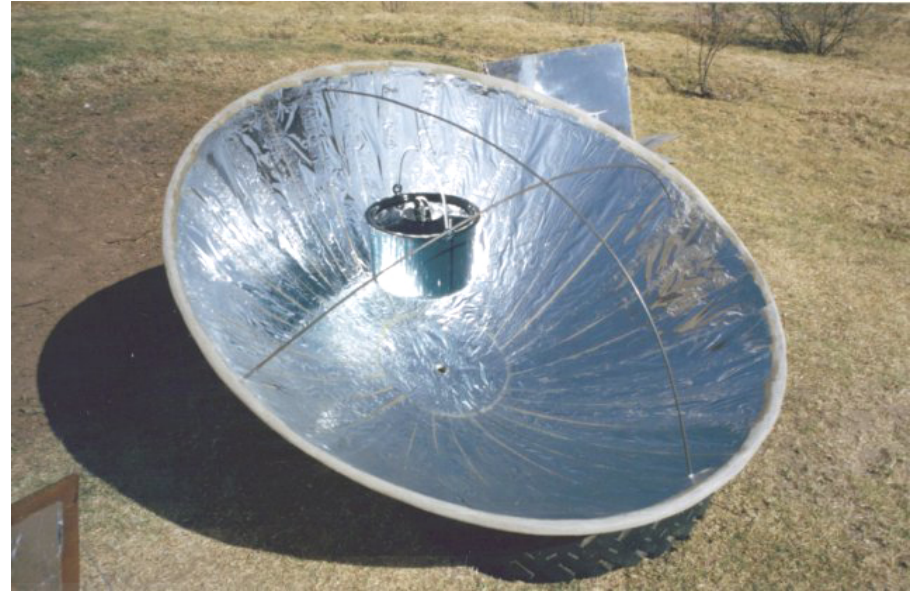
Concave solar concentrator
