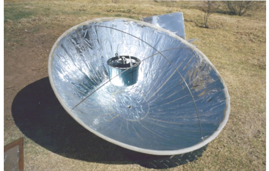
Concave solar concentrator
