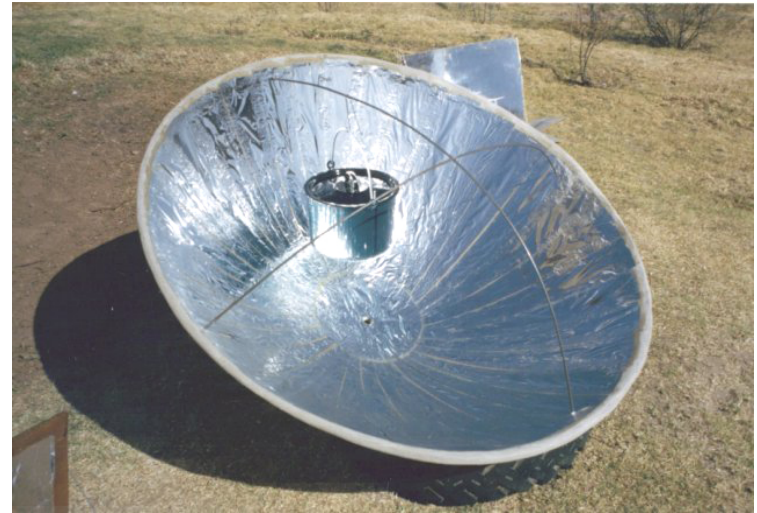
Concave solar concentrator
