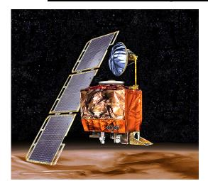
(1999) NASA lost \$125 million Mars Climate Orbiter due to Lockheed Martin giving thruster data in British units and NASA expecting metric units.
