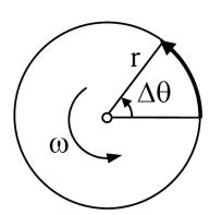
Motion of a "rigid" body about a fixed axis of rotation.
