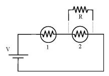
1. Predict what will happen to the brightness of each of the bulbs when you place a  $(R = 40 \Omega)$  resistor in parallel with bulb #2 as shown in the schematic. Your group should come to consensus on your predictions before doing the experiment!
