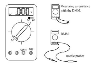
to through the device you are testing. If a power supply or battery is present in the circuit, it will add additional currents and make the computed resistance incorrect; *these additional currents can damage the meter*.
