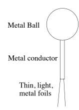
You can NOT tell what the sign of the net charge on the electroscope is simply by looking at it: If it's net +, the foils repel. If it's net -, the foils repel! So, all you can do is see how strongly charged it is, but not the sign itself.
