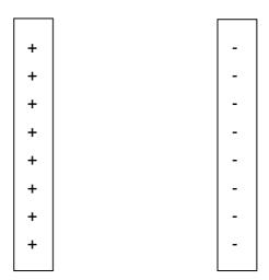
C. A positive charge is placed at position A between the two plates. State the increase/decrease in potential energy of the charge if it is moved from (a) A to B, (b) B to C and (c) C to D. How large is the work to be done to move a charge along an equipotential curve?
