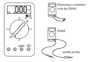
second wire is attached to the " $V\Omega$ " (volts & ohms) input. In this lab, all your measurements will be DC, so the DC/AC switch (upper right) should always be in the DC position. The DMM has an alarm; it rings if you have wires plugged into positions which conflict with the central knob's position. The 2 wires attached to the DMM are called "needle probes". You can quickly measure the difference in voltage between any two points in a circuit by touching the points with the needle probes.
