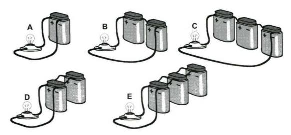
Draw the equivalent circuit diagram for each of the circuits A - E. For each of the five circuits *predict* the voltage difference across the bulb, assuming each battery has voltage of 6 V.
