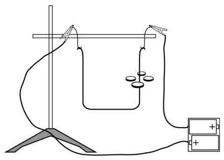
The direction of the magnetic field around a current-carrying wire can be determined by the **right-hand rule**. Namely, if you point your thumb in the direction of the current, your fingers will curl in the direction of the magnetic field lines which surround the current. In other words, the direction of the magnetic field around a straight wire carrying a current is a series of circles with a direction that follows the direction of your fingers.
