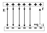
Consider 2 charged parallel metal plates (called a "capacitor"), a fixed distance d apart.
