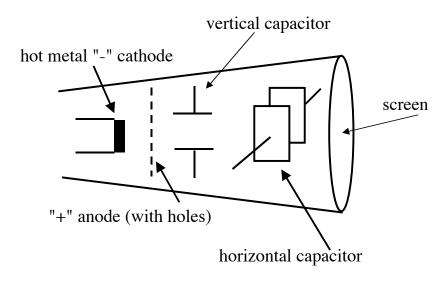
A "cathode ray" is an old-fashioned name for electrons. The "cathode" is a heated piece of metal, set at a very low voltage. The "anode" is set at a high potential (so the "cathode" and "anode" basically form a capacitor) Electrons boil off the hot cathode, and then they are accelerated towards the high voltage ("+" charged) anode. The anode is a grid with lots of holes, so many electrons can fly right on by and cruise towards the screen.
