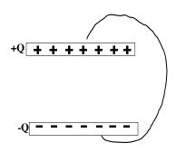
If you connect a wire up to a capacitor (like on the left) the charges on the capacitor plates are free to travel. The + and - attract one another, the capacitor will discharge quickly, possibly with some nice sparks. There's energy in there!
