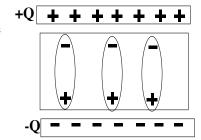
The net effect is that E is reduced throughout the dielectric. And since V=Ed, the voltage between the plates is reduced.
