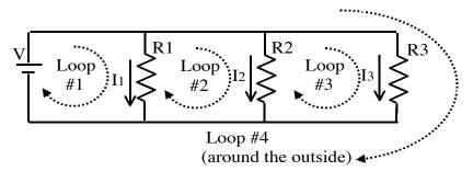
Look at the loop labeled #1. You can start wherever you want, let's begin at the bottom and imagine "walking around" the loop in the direction shown. We first go UP the battery (voltage change +V), and then we go DOWN the resistor R1, with voltage change -I1\*R1. It's a drop - think hard about every minus sign here:
