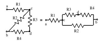
If I asked for the "equivalent resistance" between a and b in the
