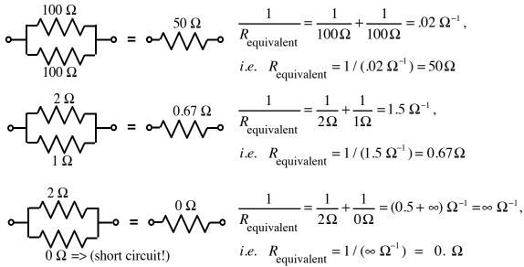
(The last is a short circuit, 0 resistance. All the current is happy to flow through the 0  $\Omega$  side!)
