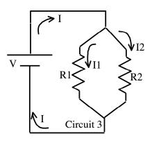
This time, the current I is NOT necessarily the same through R1 and R2.
