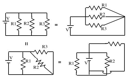
All those circuits are just 3 resistors in parallel. I personally prefer the first drawing, because it makes it visually obvious that the voltage V across all 3 resistors is exactly the same. (Like 3 parallel runs down the ski hill) By the way, this setup is pretty much how houses are wired up for appliances: here's one MORE drawing, which is pretty much equivalent to all the ones above:
