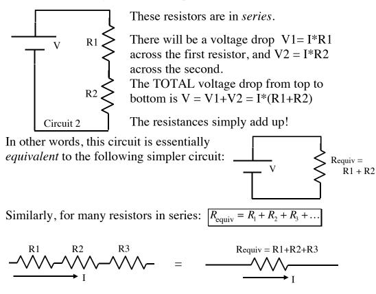
*Important:* the current I is the SAME through each of these series resistors. (What goes in must come out: conservation of charge! This is not an approximation of any kind, it's exactly true)
