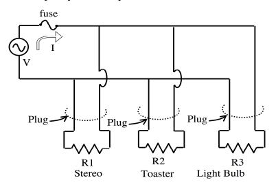
(V=120 V AC, the fuse shuts off current to all 3 appliances if I exceeds about 15-20 A)
