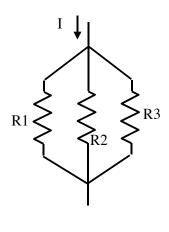
$\frac{\overline{R_{\text{equivalent}}} = \overline{R_1} + \overline{R_2} + \overline{R_3} + \dots}{R_2 + \overline{R_3}} + \dots}$ We can prove it mathematically (if you're interested): It comes from the fact that I = V / R<sub>equiv</sub>, but conservation of charges (current) says  $I = I_1 + I_2 + I_3 + \dots = \frac{V}{R_1} + \frac{V}{R_2} + \frac{V}{R_3} + \dots$  $= V * \left(\frac{1}{R_1} + \frac{1}{R_2} + \frac{1}{R_3} + \dots\right) = V / R_{equiv}$
