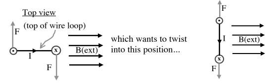
Note what happened: that loop had its *own* little B field (I didn't draw it, because it would clutter the diagram, but it points into the page in the figure at the top) originally. After it twists, that internal B field (which I still haven't drawn, but you can figure it out-) now points the *same direction* as the big B external!
