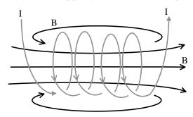
Each loop makes a B like the one on p. 20-6, and these *superpose*.
