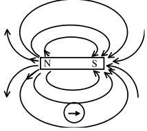
Remember, opposites attract, and a compass needle's tip is (by definition) "N", so the compass points towards (is attracted to) the "S" pole of other magnets.
