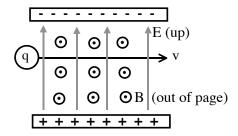
Imagine having both **E** and **B** fields together in one place. E.g, picture a capacitor (with a big **E** field) inside a magnet whose **B** field was perpendicular to **E**.
