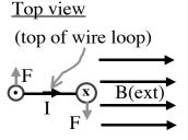
As shown, the loop starts to twist. Suppose, when the loop just reaches its "equilibrium" position, (the orientation where it feels no more net twist, or torque...)
