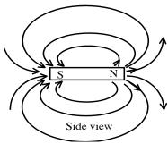
Indeed, that's basically what a bar magnet is like, microscopically, The wire loops, however, are not connected like in the solenoid- they are little circular atomic currents!
