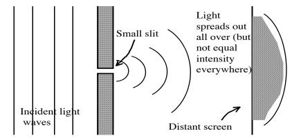
The lines I drew are NOT the same as in the previous picture, they are not "rays". Now we're trying to indicate the wave nature by drawing "wavefronts". You might think of this as connecting points where |E| is cresting. These lines are now *perpendicular* to the direction of travel of the waves. (Think of it as looking down at waves on the ocean, and what I'm drawing is the lines where the waves are highest) In the picture above, the waves move right.
