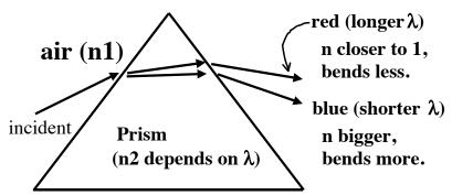
Notice that the spread of colors is *opposite* the way it goes with a grating. (In a grating, red has longer wavelength, and so bends more. In a prism, red has smaller "n", so it bends *less*.) The mechanisms involved are really totally different.
