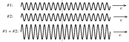
If they are "in phase" (meaning, the peaks are lined up) and if the waves are traveling at the same place and time, they will add up, they **superpose**, as waves always do. The resulting wave, the sum of the two, has the same f, c, and direction, but *twice* the amplitude. The waves have **constructively interfered**.
