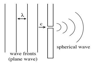
Each point on *any* wavefront can be considered to be the source of a new outgoing spherical wave.
