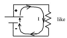
This is NOT like discharging a capacitor (where the flow is quick, and then stops when the capacitor is discharged). The battery keeps maintaining a constant voltage difference, the current is continuous.
