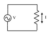
The squiggle on the left is the symbol for an AC voltage source, rather than a battery.
