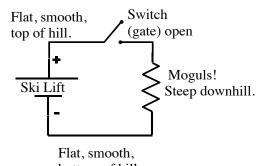
I added a new circuit element here, a switch. As shown, it's "don't pass",
