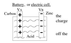
That means the carbon side is now at a *higher potential*, VA > VB. (Right? It's always higher voltage near the + charges, remember that?) This potential builds up, but if VA gets *too* high, the acid can't pull electrons off any more (the electrostatic attraction of e-'s back onto the + carbon rod will equal the chemical attraction of the e-'s into the acid)
