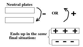
Our convention is always to define current I as the flow of imaginary "+" charges. (Even if in *reality* it's really negatives going the other way. In most conductors, it really *is* negative electrons flowing opposite the current.)
