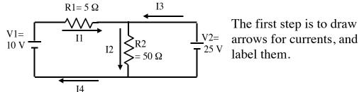
The direction you initially pick for the arrow is arbitrary! It doesn't matter. If you solve for, say, I1 in the picture above, and if it happens to come out negative, that just means the real current is heading the OPPOSITE way from the arrow you drew. (So, it'd be left, in the picture above.)
