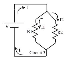
This time, the current I is NOT necessarily the same through R1 and R2.
