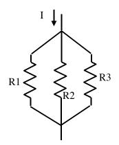
$$\frac{1}{R_{\text{equivalent}}} = \frac{1}{R_1} + \frac{1}{R_2} + \frac{1}{R_3} + \dots$$
