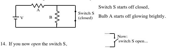
what happens to the brightness (which really means the power) of bulb A?
