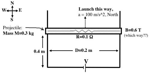
A battery (voltage "V") drives a large current around a closed metal loop composed of fixed rails and a conducting bar (that's the projectile, it has length D=0.20 m, and mass M=0.30 kg) which rests on the rails a distance 0.40 m from the battery.
