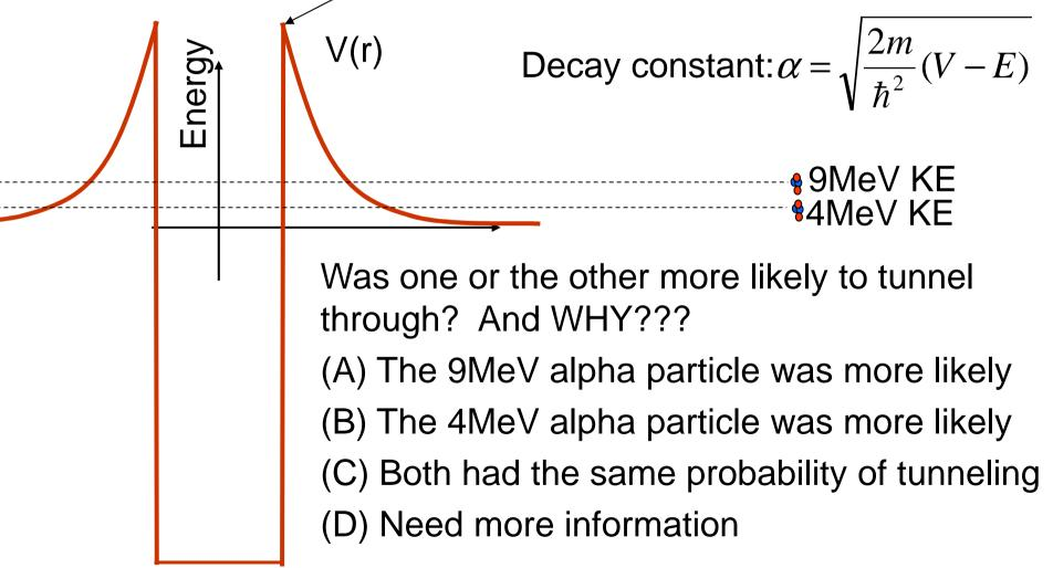
Observe a particles from <u>different isotopes</u> (same protons, different neutrons), exit with different amounts of energy.
