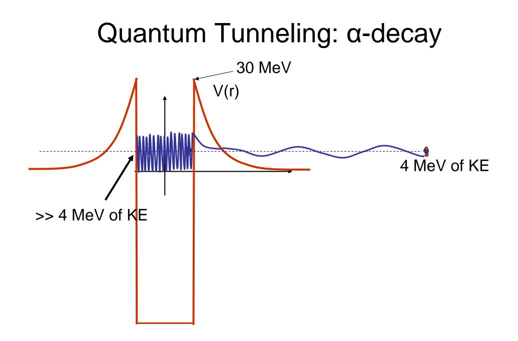
Observe α-particles from <u>different isotopes</u> (same protons, different neutrons), exit with different amounts of energy.
