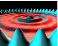
Here they have positioned 48 iron atoms into a circular ring in order to "corral" some surface state electrons and force them into "quantum" states of the circular structure. The ripples in the ring of atoms are the density distribution of a particular set of quantum states of the corral - IBM Research
