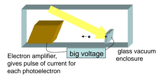
Apparatus to detect single photons (eye is incredible good: can detect few photons)
