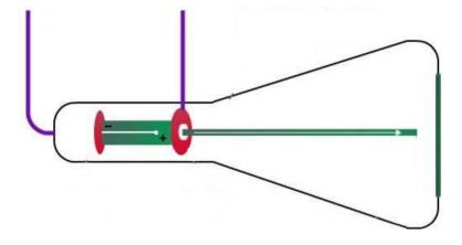
E-field: ray consists of charged particles
