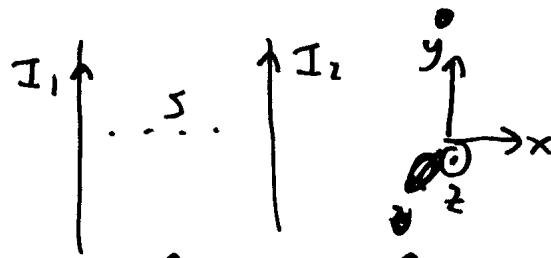
$$\mathbf{B}_{\text{due to } I_2} = \frac{\mu_0 I_2}{2\pi s} \text{ into page } (-\hat{z} \text{ direction})$$
