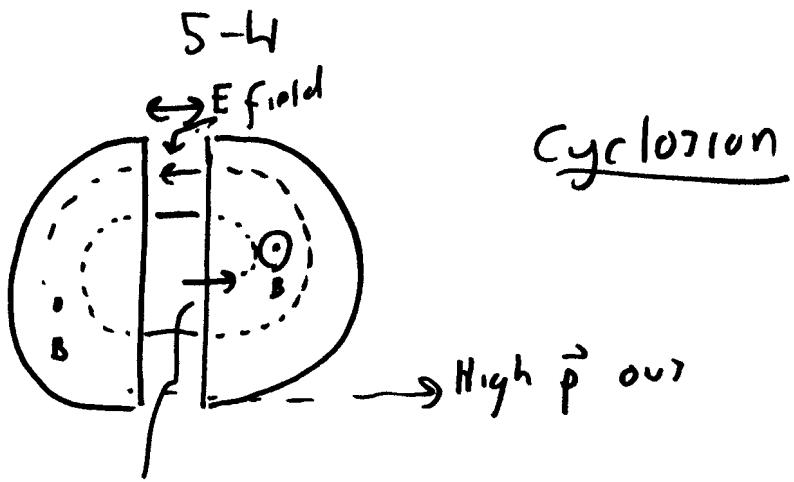
inject low  $\vec{p}$  electron, fixed time  $T_{1/2} = \frac{1}{2f} = \frac{qB}{4\pi m}$  to go
