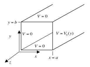
In order to find out the voltage inside the pipe, you will need to solve Laplace's equation:
