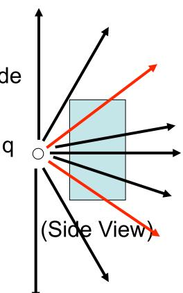
A Gaussian surface which is *not* a sphere has a single charge (q) inside it, *not* at the center. There are more charges outside. What can we say about total electric flux through this surface  $\oint \vec{E} \cdot d\vec{a}$ ?
