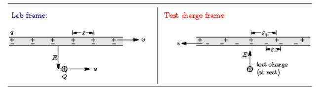
Shown above is a model of a wire with a current flowing to the right. To avoid minus signs we take the current to consist of a flow of positive charge carriers, each with charge +q, separated by an average distance of  $\ell$ . The wire is electrically neutral in the lab frame, so there must also be a bunch of negative charges, at rest, separated by the same average distance  $\ell$  in this frame. (Be aware that charge is Lorenz invariant: a charge Q has the same value in every inertial frame.)
