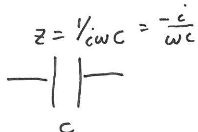
General procedure: Pretend you have a simple resistor circuit, using  $Z$  in place of  $R$ , and solve for  $V, I$  using usual phys 1120 (Kirchoff or "reducing equivalent resistors") methods.
