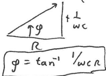
$$\text{tells me } e^{i\phi} = \frac{R}{\sqrt{R^2 + \frac{1}{\omega^2 C^2}}} + \frac{i/\omega C}{\sqrt{R^2 + \frac{1}{\omega^2 C^2}}}$$
