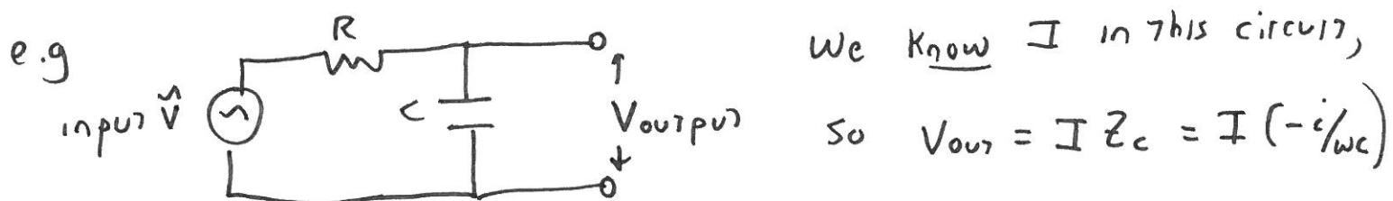
$$\text{thus } V_{\text{out}} = \frac{V_{\text{in}}}{R - \frac{i}{\omega C}} \cdot -\frac{i}{\omega C} = V_{\text{in}} \cdot \frac{1}{1 + i \omega R C}$$
