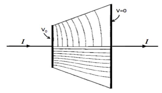
**D.** The diagram now shows the <u>correct</u> *equipotential* lines (upper half) and <u>correct</u> *E-field* lines (lower half) inside this cone-shaped resistor.<sup>1</sup>
