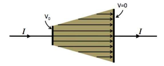
**B.** For this same situation, the diagram now shows one way that a student has drawn the electric field lines inside the resistor.
