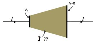
In the figure, predict (sketch) the E-field lines inside the resistor.
