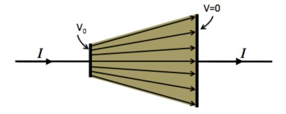
**C.** The diagram now shows another way that a student has drawn the electric field lines inside the resistor.
