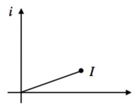
Given  $V = V_0 \exp(i\omega t)$  and  $Z = 2\exp(-i\pi/2)$ , plot the complex number I = V/Z at the instant in time shown in the diagram below.
