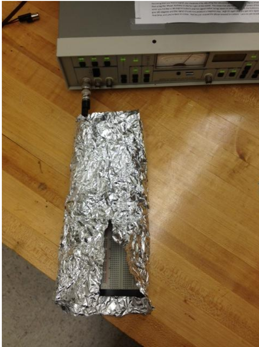
Figure 8.6 Circuit board wrapped in an aluminum foil shield. Connect the shield to ground with an alligator clip. Be careful that the shield is not shorted to any other wires in your circuit.
