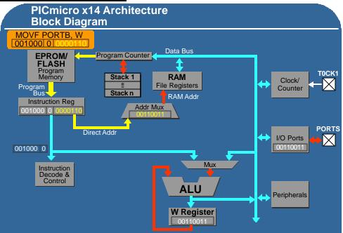
This completes this particular instruction, but to look at the remainder of the block diagram, you can see all the peripherals including the timers, clocks and counters sit on the same data bus, although they all have different addresses.
