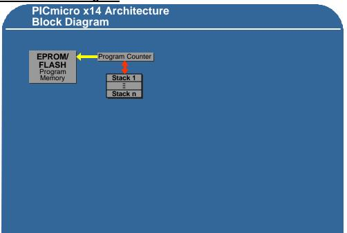
Let's now take a look at the block diagram of the PICmicro x14 architecture starting with the program memory space. EPROM memory or Flash EEPROM program memory space is addressed from the program counter. The program counter on the x14 architecture is 13 bits long.
