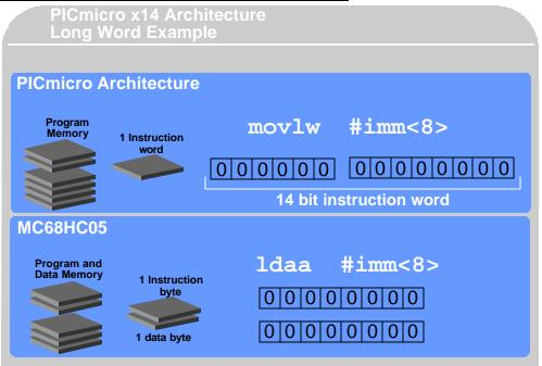
This shows an example of the Long Word Instruction, the MOVLW #IMM, which loads the immediate value designated here as #IMM into W. In this architecture, the immediate value is always an 8-bit number. You can see the constant here is 8-bits so we can store 8-bit immediate values in the 14-bit wide instruction word. The 4-bits used for the op-code in this case, MOVLW, translate into 1100b.
