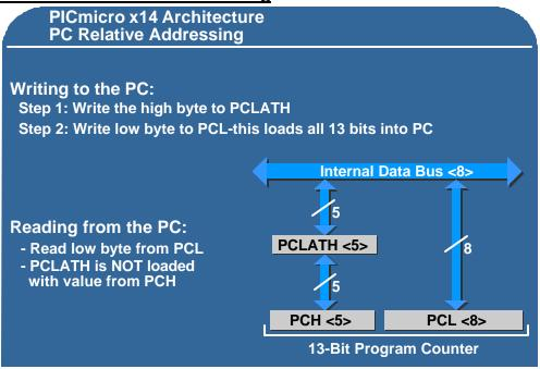
Lets go through the steps required to write to the program counter when using relative addressing.
