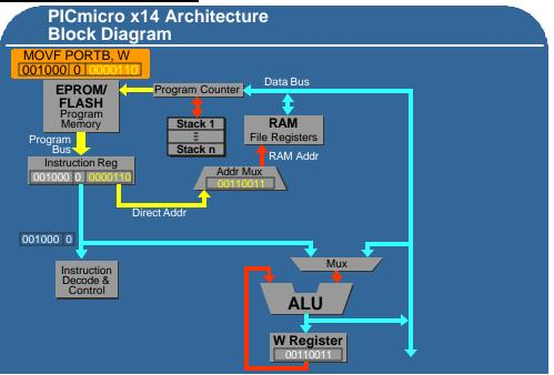
In this case the top 7-bits of the instruction are decoded and tell the processor that it needs to do a move-file instruction and put the result in the W register. The address goes into the address multiplexer and since we are using direct addressing in this example, PORTB is used to address the RAM or the file register space. Notice the W register is a part of the ALU on the x14 architecture. It does not have a separate address space in this architecture.
