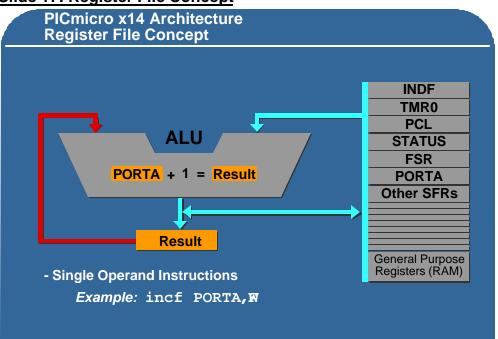
One of the features in the PICmicro architecture that makes it so powerful is the use of register files. The register file concept means that all RAM locations, peripherals and I/O ports are organized as a simple bank of registers. All instructions can operate on any register and you don't have to load things from RAM into a register to do functions on them.
