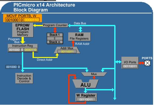
Since the I/O ports sit on the same data bus as the file registers and RAM locations, you can address I/O ports and RAM using exactly the same instructions that you would for file registers. Just change the address and the instruction will execute on the RAM location or the I/O port, because they sit on the same 8-bit data bus.
