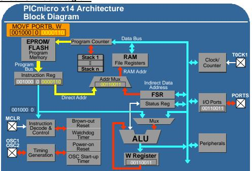
Before we leave this section, lets briefly discuss the auxiliary features that are built into the PICmicro x14 architecture. These include the brown out reset, watch dog timer, power on reset and oscillator startup timer, all of which are generic functions available in the PICmicro x14 family of products.
